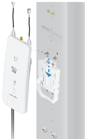
Mounting on a Sector Antenna
